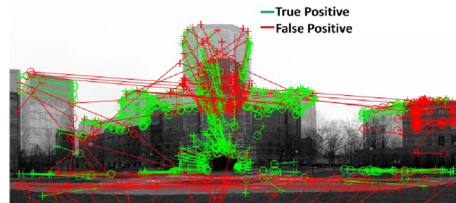
Figure 3: \mathcal{FA}_0 is highly flawed when two cameras are far apart from each other.
